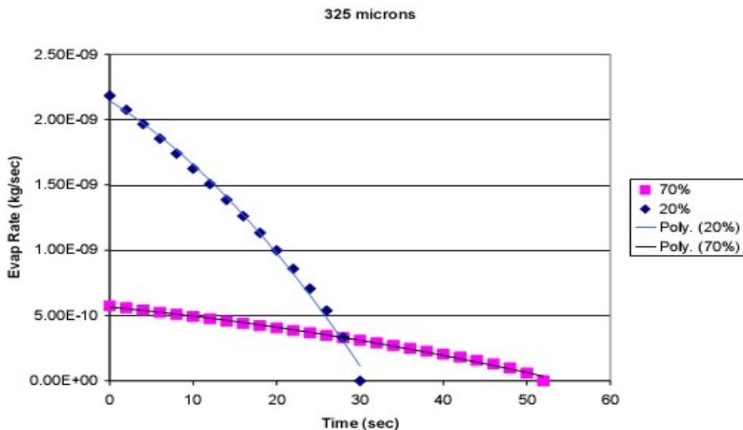
Figure 2 – The evaporation rate for a 325 micron diameter drop in an ambient air control volume, shown here against time, decreases until the drop is completely evaporated.
