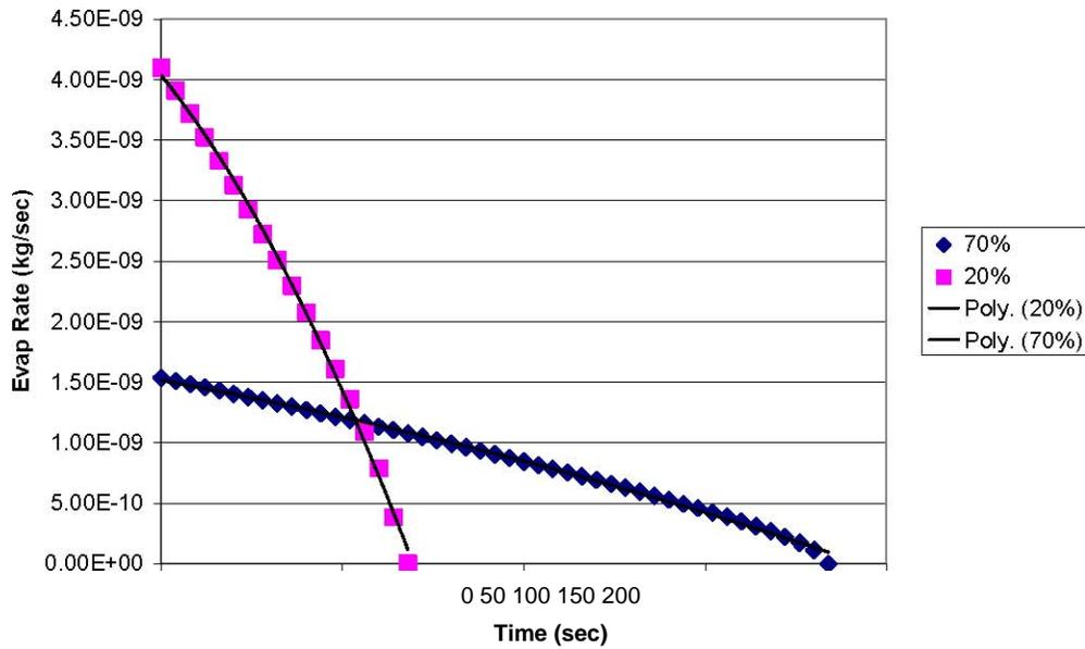
Figure 3 - The evaporation rate for a 680 micron diameter drop decreases similarly to the 325 micron drop. The evaporation rate slows as the drop evaporates until the drop is completely vaporized.
