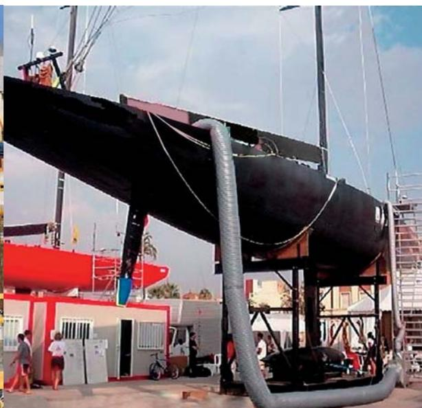
Boat drying, made by dehumidifier model EH200.
