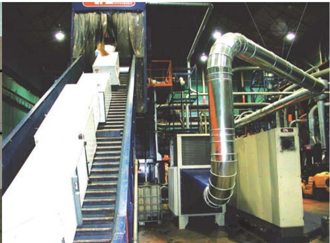
Triturating industrial plant; Humidity control in CFC's gas recovery, Required process temperature 60°C, relative humidity 30%. Dehumidification made by special unit model KSD800.
