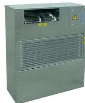
Residential dehumidification plant, combined to radiant cooling system. The dehumidifier (FH GH series) controls the latent load of the room, while the radiant cooling system manages the sensible one.
