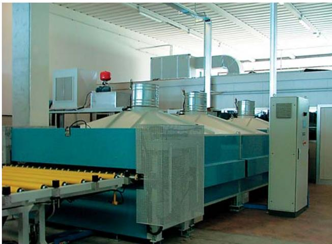
Stratified glass production plant; required temperature 18°C, relative humidity 25%, made by dehumidifier with temperature control model DS3000, airflow 3000 m<sup>3</sup>/h.
