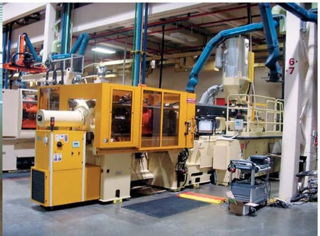
Plastic injection plant; required dew point -8°C, dehumidification made by special unit, airflow 1200 m<sup>3</sup>/h, air outlet conditions 20°C, relative humidity 10%.
