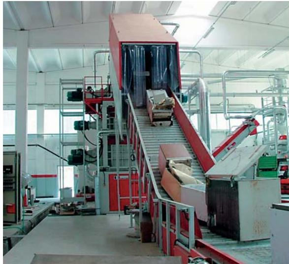
Triturating industrial plant; humidity control in CFC's gas recovery, required process temperature 60°C, relative humidity 30%. Dehumidification made by special unit model KSD800.
