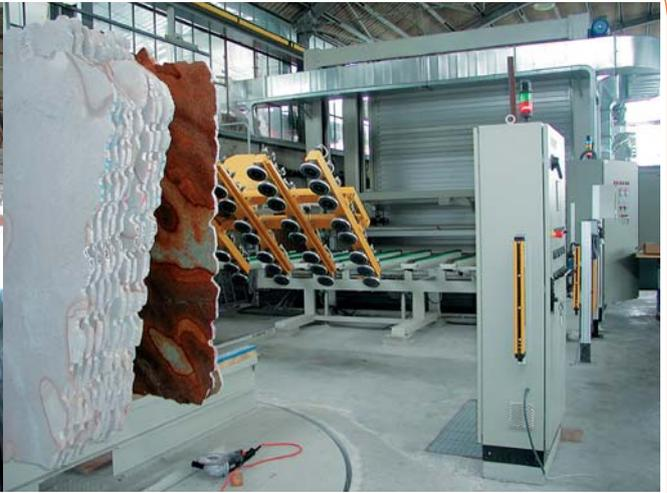
Marble resin topping plant; required process temperature 45°C, relative humidity  $\leq 15\%$ , made by dehumidifier with temperature control model KSR1500. Airflow 15000 m<sup>3</sup>/h.
